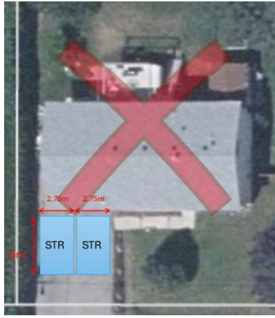
Parking spaces must have a minimum depth of 6 m
